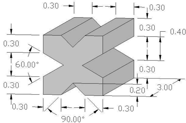
**Hint:** It is not as complicated as it looks. If your grids Graduations are set to 10 just snap to the intersections for the beginning and ending points of your lines. To set the constraint for the angles select the angled lines and the angle constraint will appear. Reference Step 19 for modifying the angle value.
