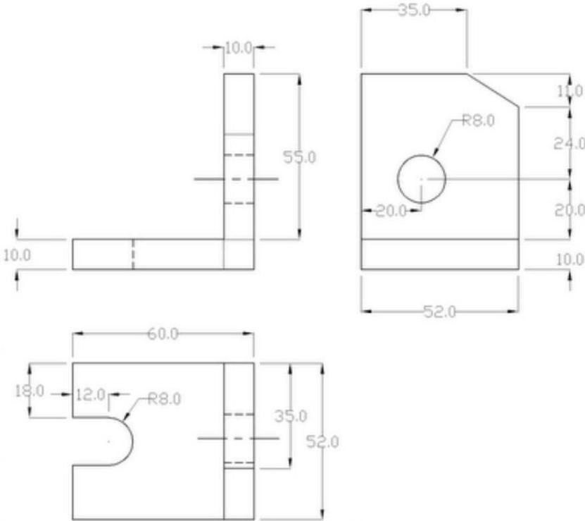
**To create a given model by Using the AUTOCAD/CATIA/CATIA**
