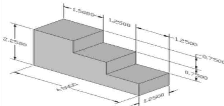
**Hint:** To help make it easier to sketch this part set the grid **Primary Spacing** to 1 and the **Graduations** to 4. This will put the grid lines in the **Sketcher** screen to .25 inch spacing. With that spacing all you have to do is snap to the intersections of the grid to sketch the part.
