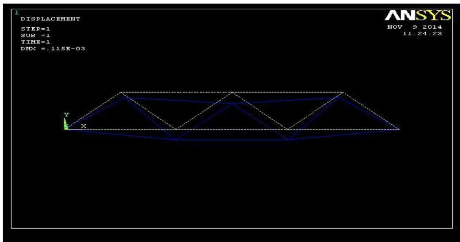
**Figure: Deformed and undeformed Model**
