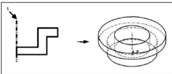
**Sweep:** Pad of a cross section along a path
