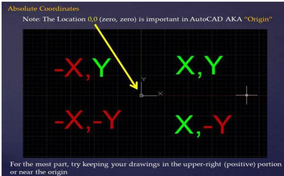
The origin is marked by an object known as the UCS icon UCS = User Coordinate System. This icon can be manipulated (moved and rotated) such that the origin point moves. But for the purposes of learning the basics of coordinates, this post will treat the UCS icon as a static object in a permanent position. Oddly enough, the UCS icon does have permanent position that it can always be re-positioned to. This position is called the "World coordinates."
