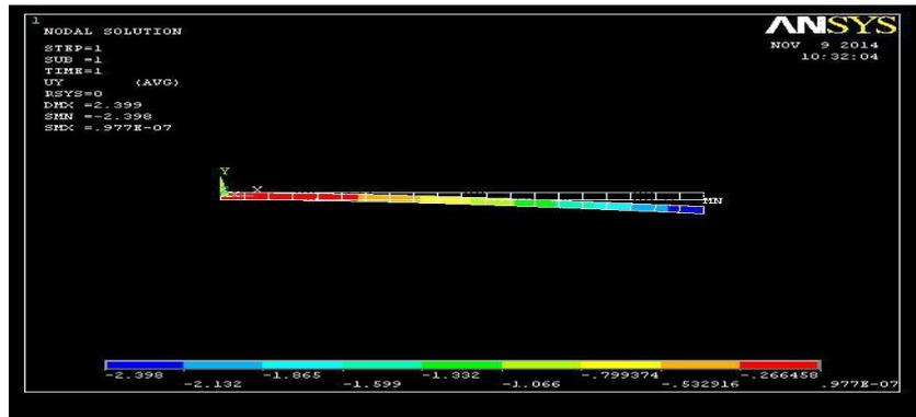
Figure: Y-Component displacement of the Model
