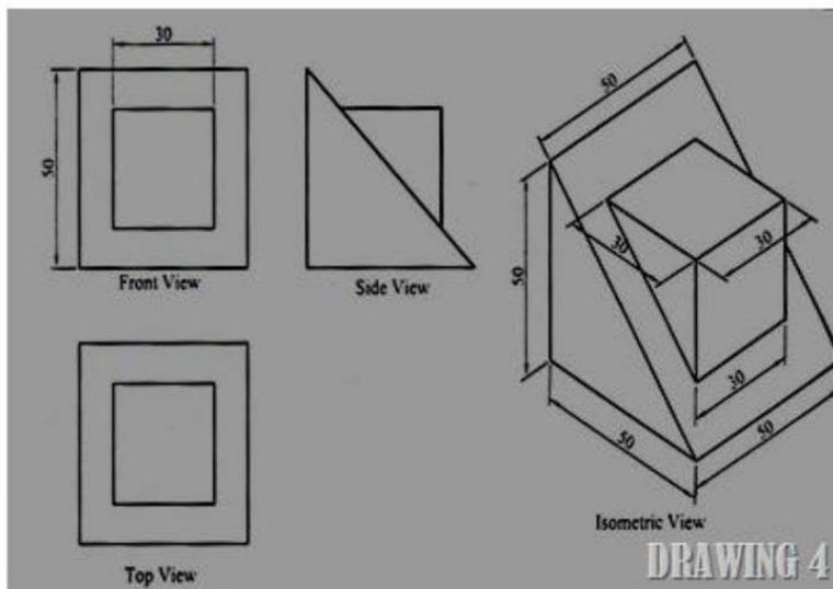
**To create a given model by Using the AUTOCAD/CATIA**
