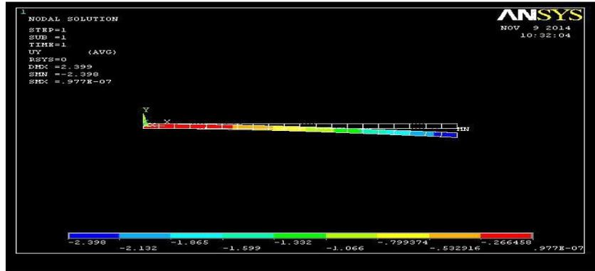
Figure: Y-Component displacement of the Model
