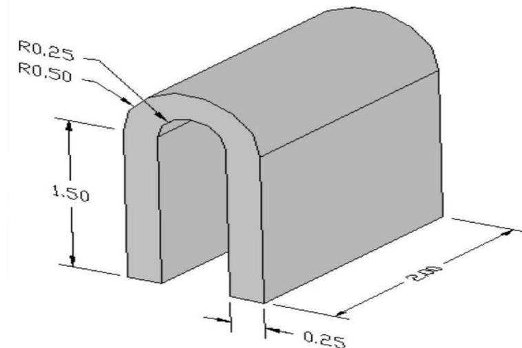
**Hint:** This part can be done using the radius option in the profile command.
