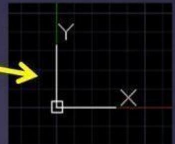
**Absolute Coordinates** let you type in a specific X and Y location on the construction plane.
