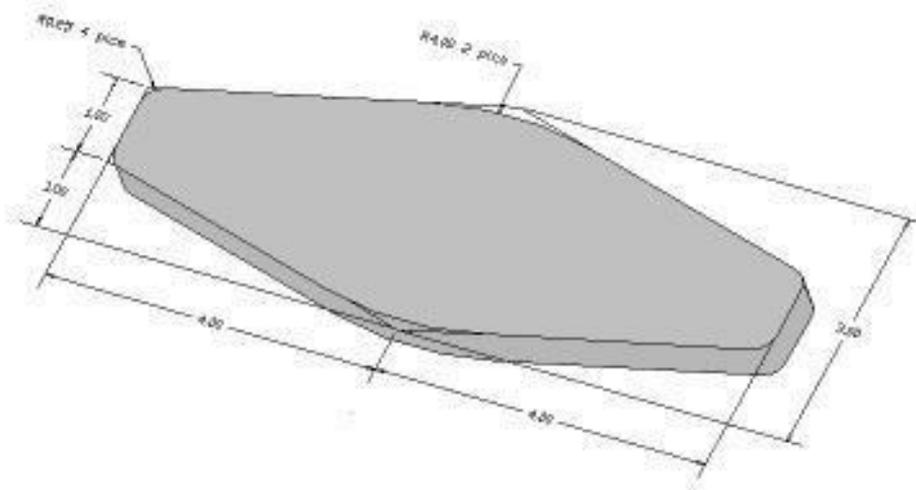
**Hint:** Use the **Line** or **Profile** icon first to sketch the profile using sharp corners (no radius). Once it is constrained to the dimensions above, go back and add in the radiuses using the **Corner** icon.
