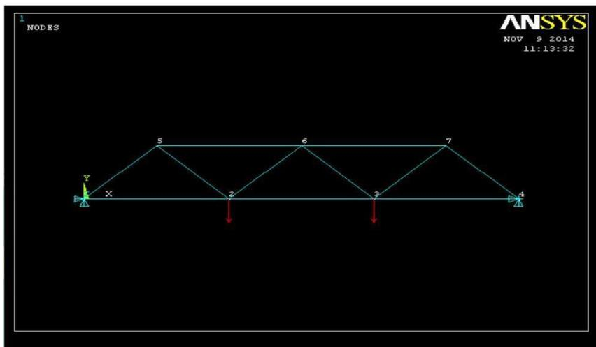
Figure: Model with boundary conditions
