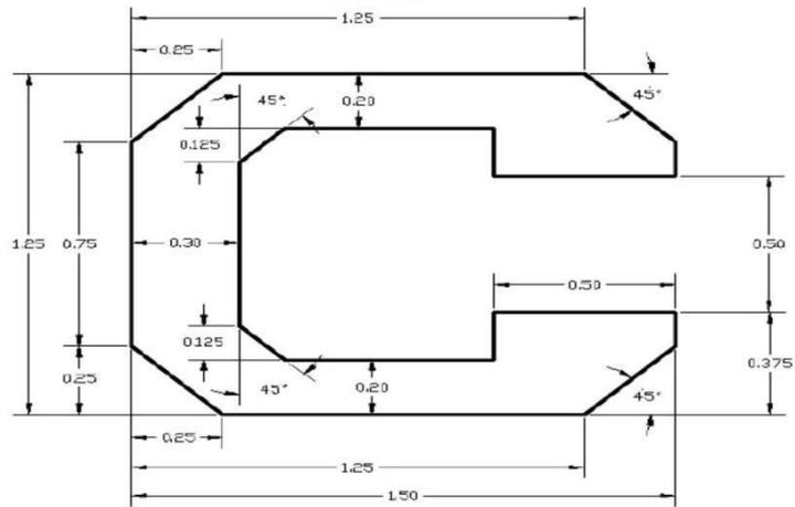
**To draw the given diagram by Using AUTOCAD/CATIA**
