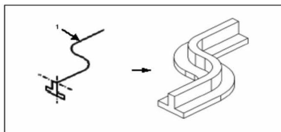
**Blend / Loft:** Blending of different cross sections along a path
