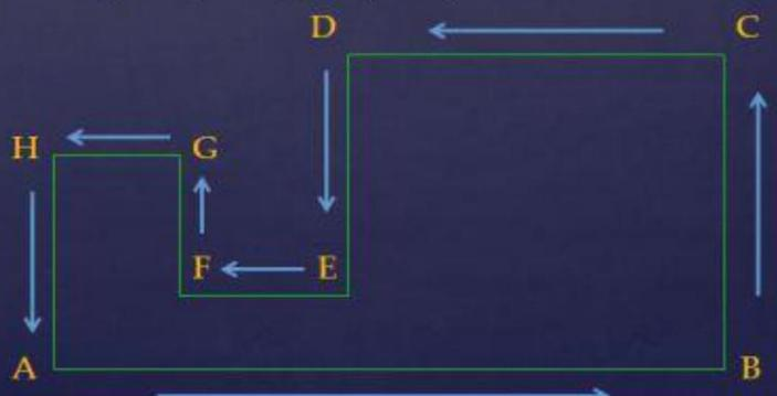
As mentioned before each exercise, Dynamic Input when enabled turns your entry method to an automatic Relative Polar method. This is confusing because when DYN is turned on and say that you want to specify the coordinate of 0, 0 you will not see anything happen. So in order to force Dynamic input to use Absolute coordinates use the # sign before the coordinates.
