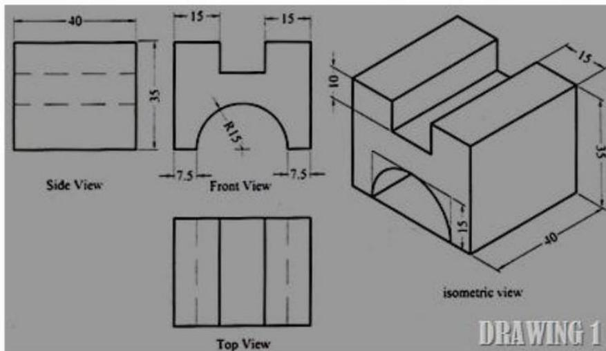
**To create a given model by Using the AUTOCAD/CATIA**
