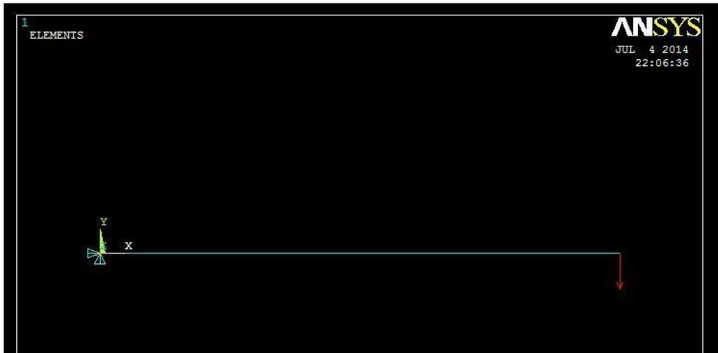
Figure: Model with boundary conditions
